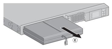
**E** - Pull the plastic tab to remove the battery block and replace it.
