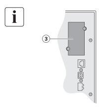
It is not necessary to shutdown the UPS before installing a communication card.
