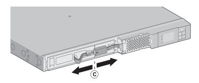
**C** - Disconnect the battery block by separating the two connectors (never pull on the wires).
