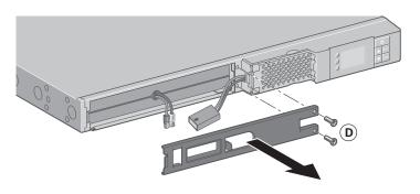
**D** - Remove the metal protection cover in front of the battery (two screws).
