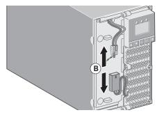
**B** - Disconnect the battery block by separating the two connectors (never pull on the wires).
