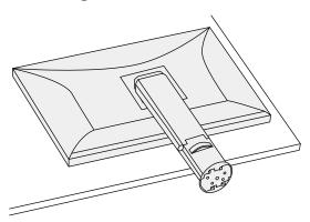
2. Hold the stand base so that the back label (FRONT) is aligned as shown in the diagram, and attach the stand base onto the stand brace.
